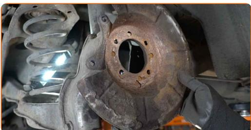
**23** Install the new wheel hub with a bearing.
