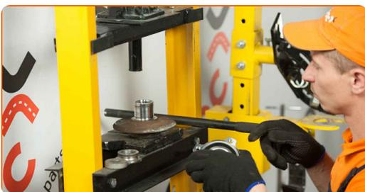
**35** Install the new wheel hub with a bearing.
